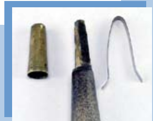
Right: Detail of trimming tool with ferrel removed and watch-spring cutter formed to desired contour.
